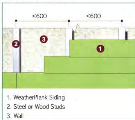
Typical siding fixing detail
