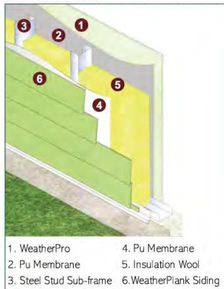
WeatherPlank siding with steel framed external wall
